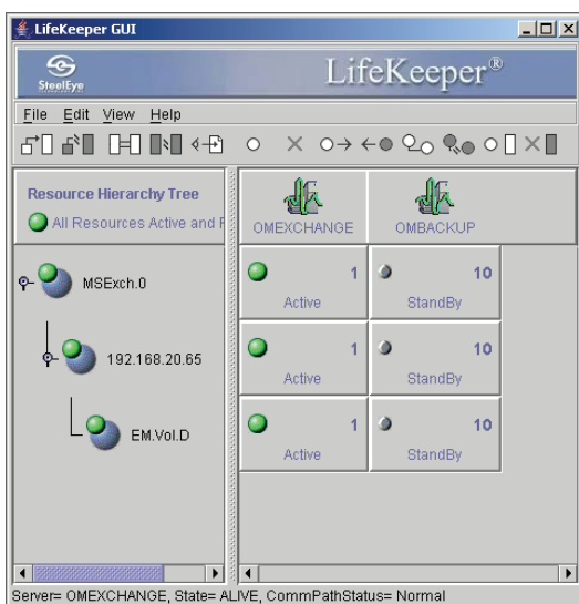
Figure 1: Once a resource has been created it can be extended to other machines in the cluster so that they can take it over if the active machine fails
